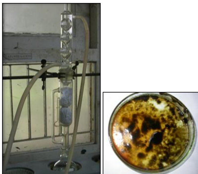
FIG. 5: SOXHLET APPARATUS AND EXTRACT
