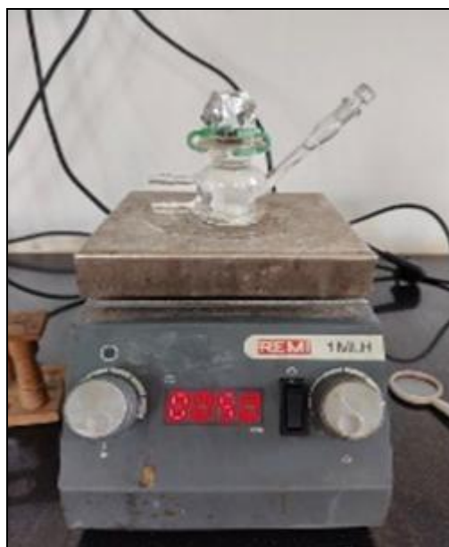
FIG. 11: FRANZ DIFFUSION CELL APPARATUS. Apparatus used for the in-vitro diffusion study.
