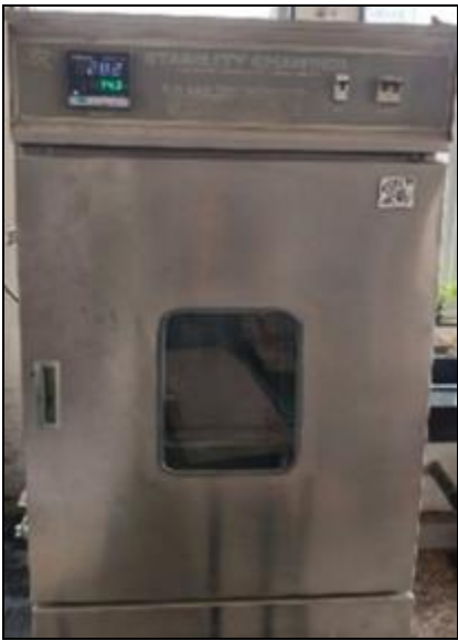
FIG. 15: STABILITY TESTING CHAMBER - Used for Accelerated Stability Studies
