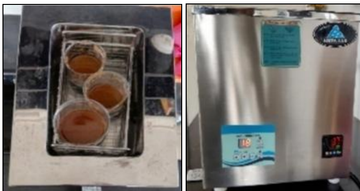
FIG. 9A AND 9B: ULTRASONICATOR USED FOR EXTRACTION. Figure shows Ultrasonicator Used for Preparation of Herbal Extracts.
