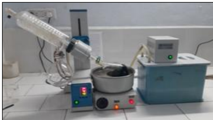
FIG. 5: EVAPORATION OF SOLVENT USING ROTARY EVAPORATOR
