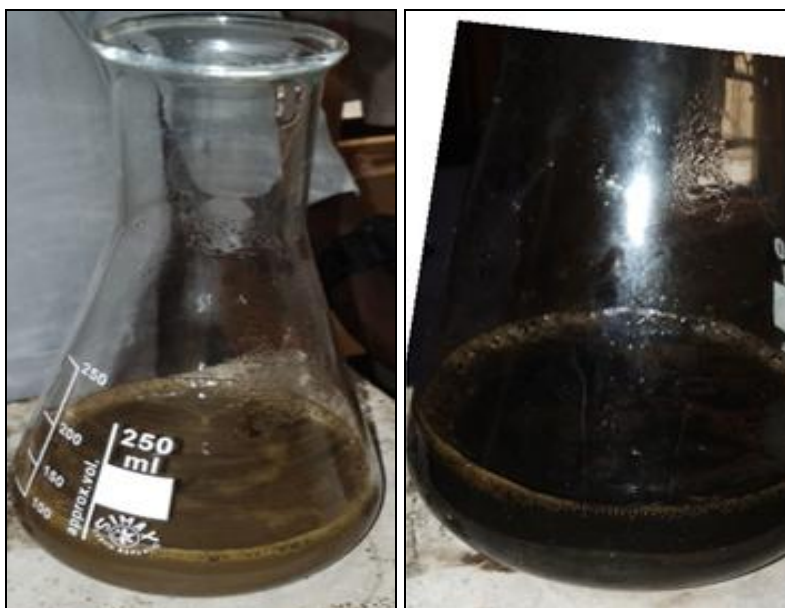
FIG. 2: AQUEOUS EXTRACT OF SENNA OCCIDENTALIS AND SYNTHESIZED AG 2 SNPS (LEFT TO RIGHT)
