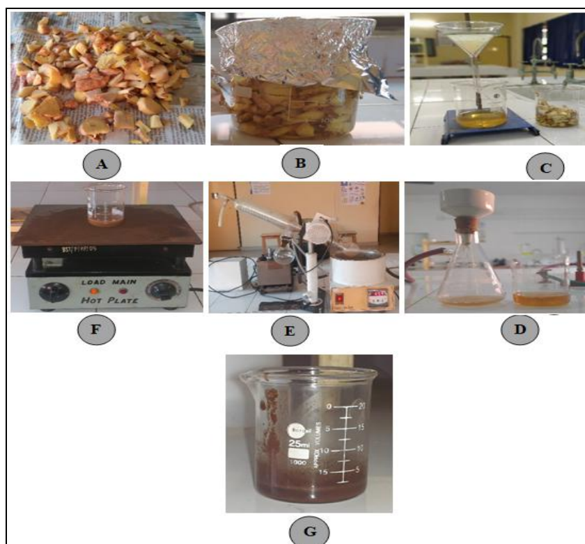
FIG. 2: EXTRACTION PROCEDURE OF ZINGIBER OFFICINALE RHIZOME (ALSO KNOWN AS GINGER)
