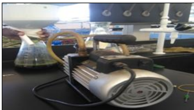
FIG. 2: LIQUID FILTER USING AN ELECTRICAL SUCTION PUMP
