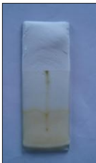
FIG. 1: TLC OF ETHANOLIC EXTRACT OF JASMINUM GRANDIFLORUM LINN. SOLVENT SYSTEM: N-BUTANOL: GLACIAL ACETIC ACID: WATER – (4:1:5)
