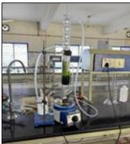
FIG. 1: SOXHLET EXTRACTION OF SPINACH OLERACEA
