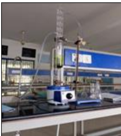
FIG. 2: SOXHLET EXTRACTION OF MURRAYA KOENIGII
