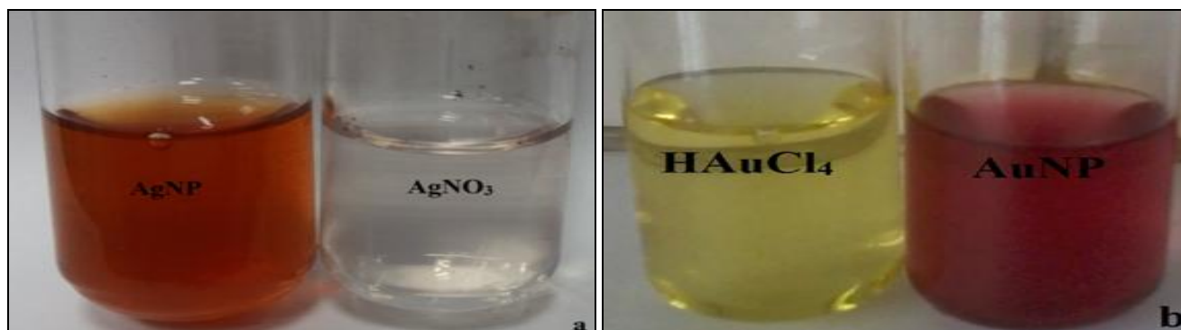
FIG. 1: A CHANGE IN THE COLOR OF REACTION MIXTURE AFTER SYNTHESIS OF AgNP (A) AND AuNP (B) BY ADDING STEM AQUEOUS EXTRACT OF ALHAGI MAURORUM TO AgNO 3 AND HAuCl 4 RESPECTIVELY
