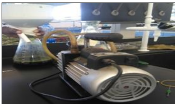
FIG. 2: LIQUID FILTER USING AN ELECTRICAL SUCTION PUMP
